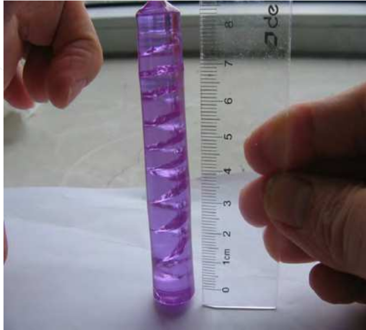
Fig. 2.1 The cracking \text{Nd}^{3+}:\text{NaY}(\text{WO}_4)_2 crystal.
