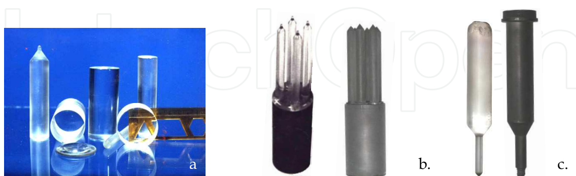
Fig. 2. (a) Calcium fluoride crystals; (b) multiple type crucible; (c) crucible with seed.
