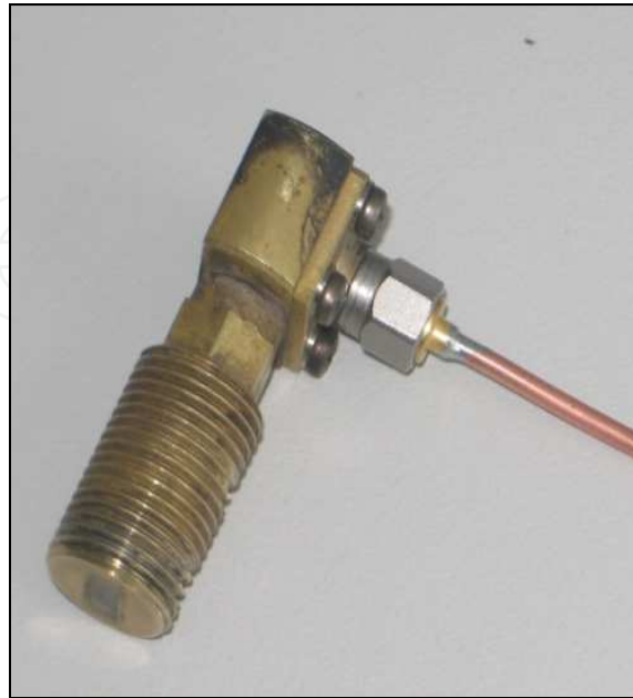
Fig. 20. The antenna for the PIT microwave sensor
