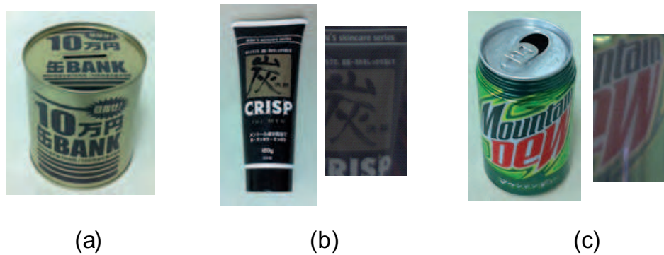
Fig. 13. Examples of object segmentation failure. (a) Object which could not be extracted. (b)Left: Object Right: Results of segmentation. (c)Left: Object Right: Results of segmentation.
