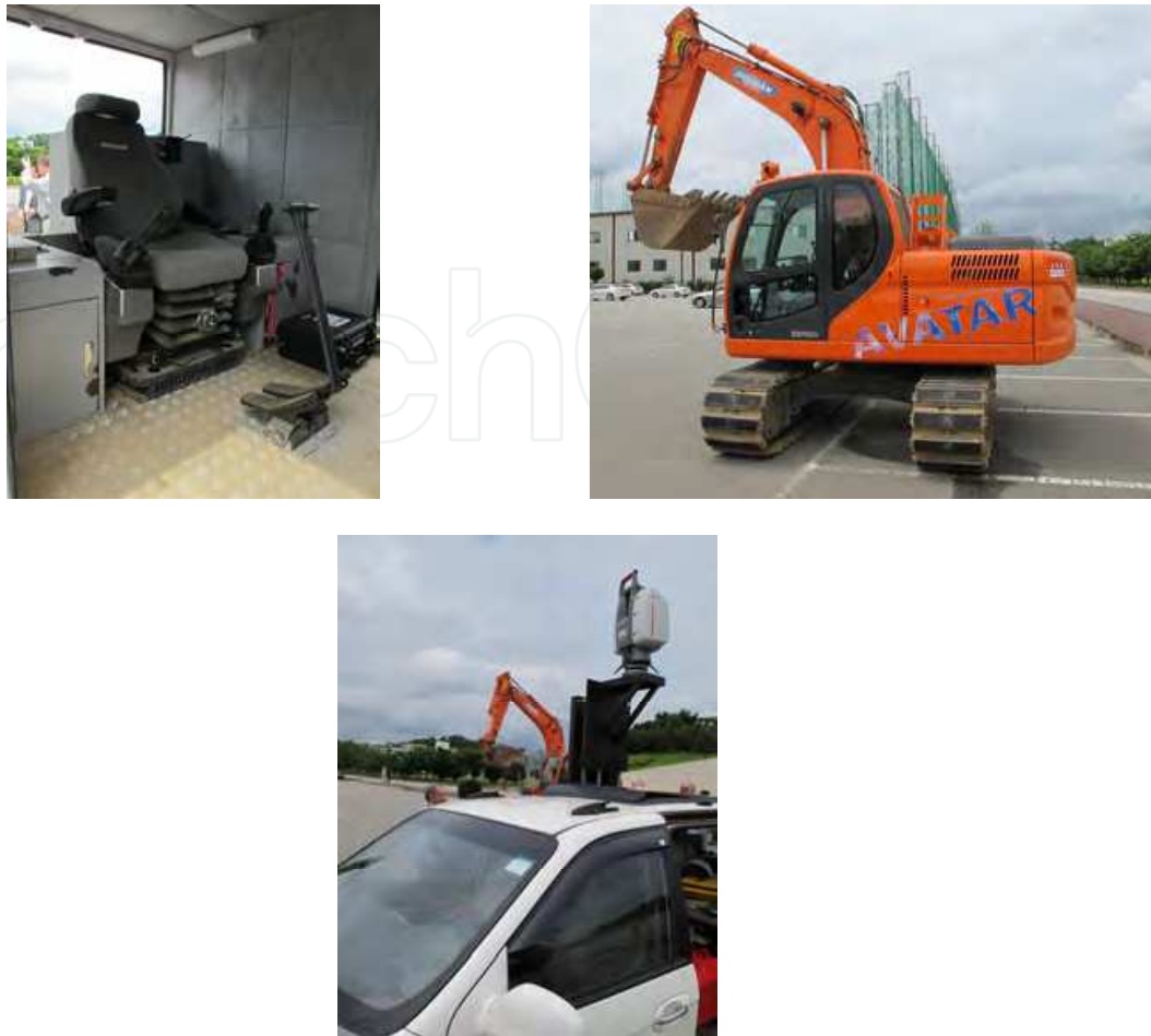
Fig. 5. Fully functioning system for tele-operation of robotic excavators, the excavators can operate on a high level of autonomy; the excavation process is monitored by separate laser module (picture right side) providing information to the robotic excavator. Hanyang University, Korea, 2011.
