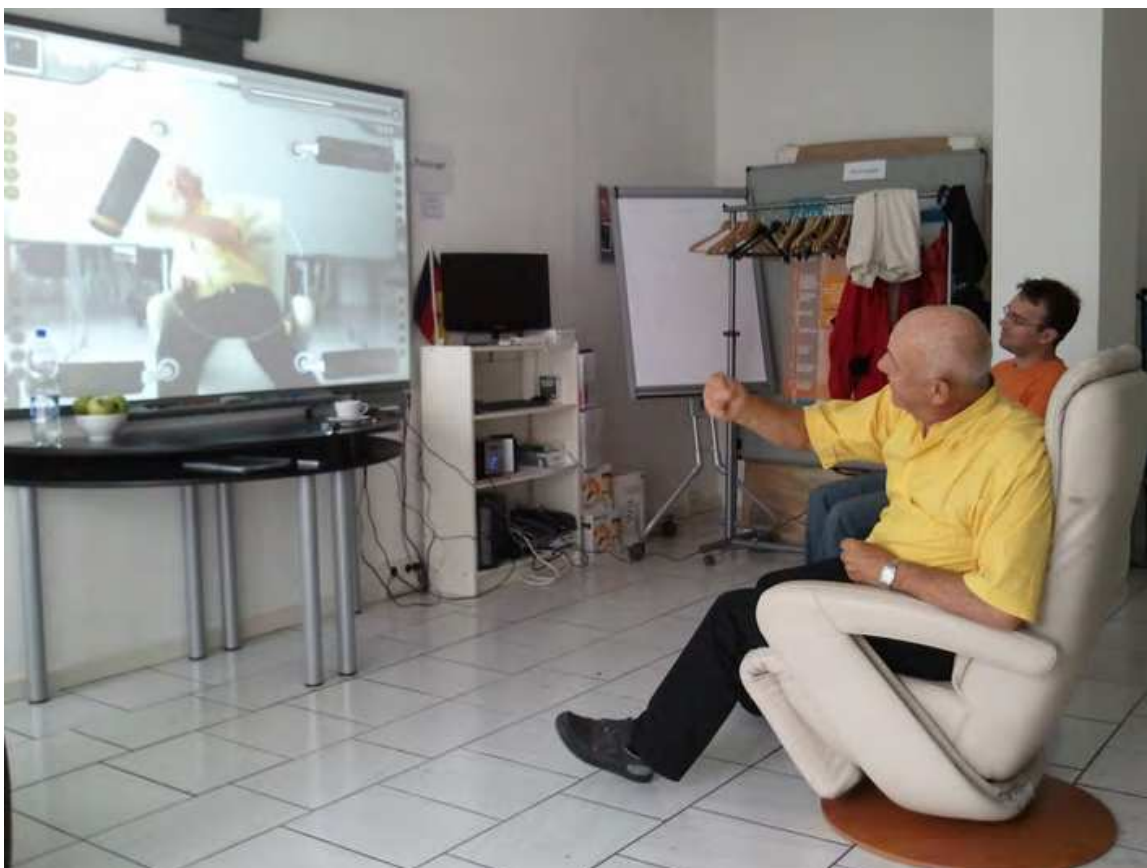
Fig. 18. Sensor Chair developed within the authors' R&D (Research & Development) Project GEWOS. The "Fitness Chair" is measuring people's vital signs, makes those vital signs then transparent to the user and finally try's to activate the user to become more active, do sports and meet friends.
