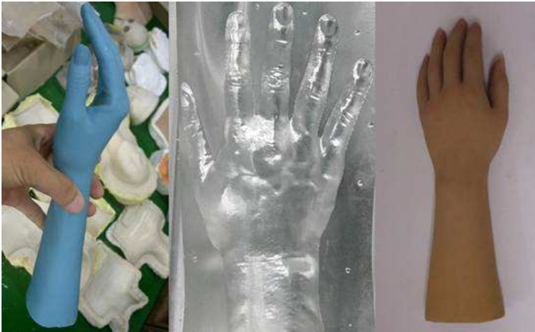
Fig. 10. The mock-up, mold and finished artificial hand skin
