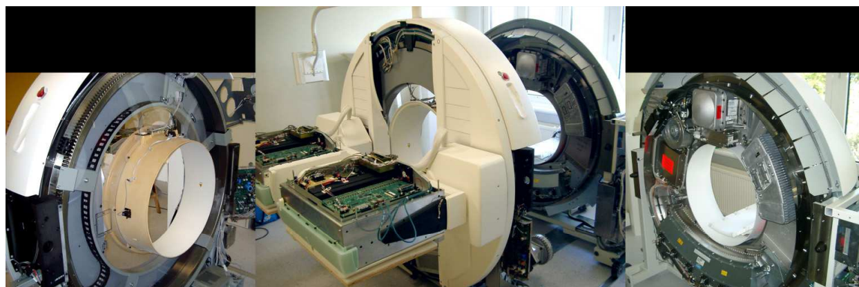
Fig. 3. Siemens Symbia T6: Left: Gantry of the dual head gamma camera, Center: both parts separated during service, Right: Gantry of the 6 slice MD CT
