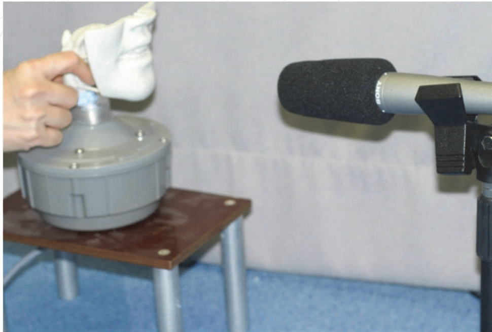
Fig. 13. Examination of analysis of vocal tract transmission characteristics using a model that was rapid-prototyped by our proposed method.
