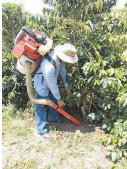
Fig. 1. Vacuum machine prototype to collect coffee berries from the ground.
