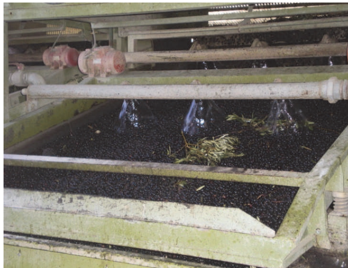
Fig. 2. Washing step for olive fruit.
