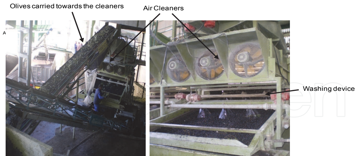
Fig. 1. Cleaning steps for olive fruit.
