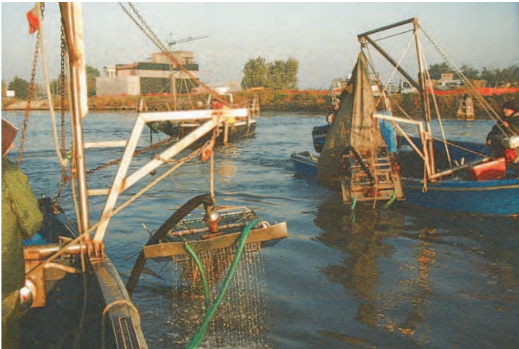
Fig. 9. Hydraulic clam dredge “idrorasca”
