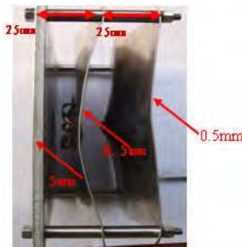
Fig. 27. Experimental result of flyer impact multi-layer structure
