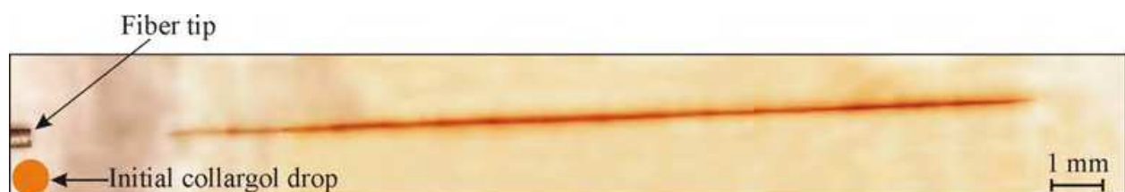
Fig. 18. Micro-image (in transmission mode) of filament of Ag nanoparticles fabricated in water nearby optical fiber tip at 2.5 W of laser power (Yusupov et al, 2011b).
