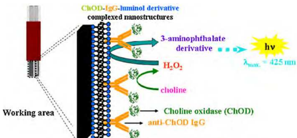
Fig. 29. Reagentless detection principle of choline oxidase activity by ECL reaction triggered directly in the sensing layer (Reproduced from Jiao et al., 2010, Colloids and Surfaces A: Physicochemical and Engineering Aspects , 354, 284-290).
