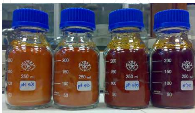
Fig. 9. Resorcinol-formaldehyde organic xerogels prepared from precursor solutions with different pHs: from left to right 5.8, 6.0, 6.2 and 6.5.
