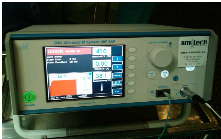
Fig. 1. RF generator: OWL universal RF System URP-3AP
