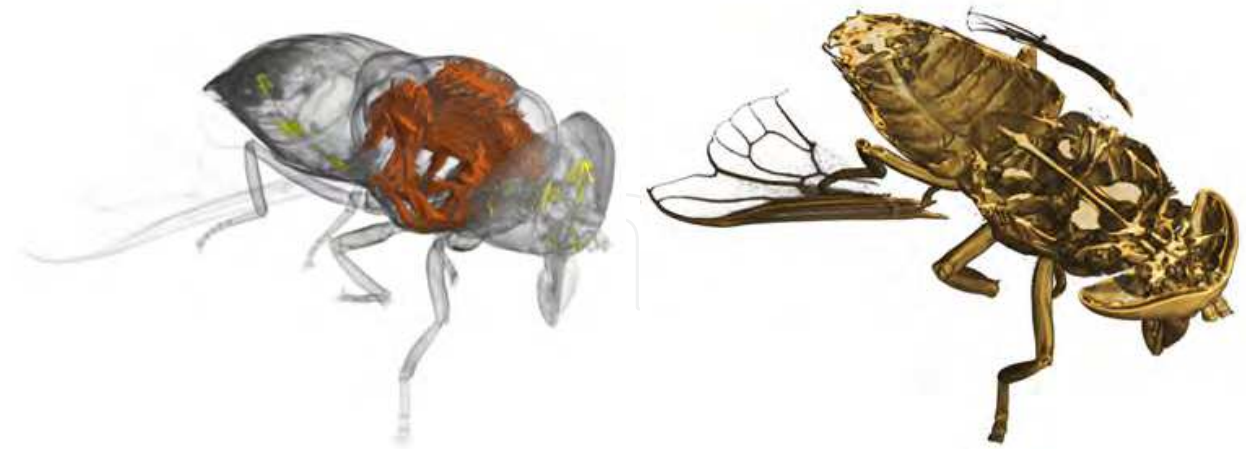
Fig. 1. Neutron tomography of a dried horsefly. Top right: outer surface, top left: upper portion sliced away, bottom right: mid-level slice, bottom left: contour of wing muscles. Note that the insect is approximately 1cm in length head to tail. Images courtesy of Dr. Eberhard Lehmann using the ICON beamline, SINQ, Paul Scherrer Institut, Switzerland 23 .
