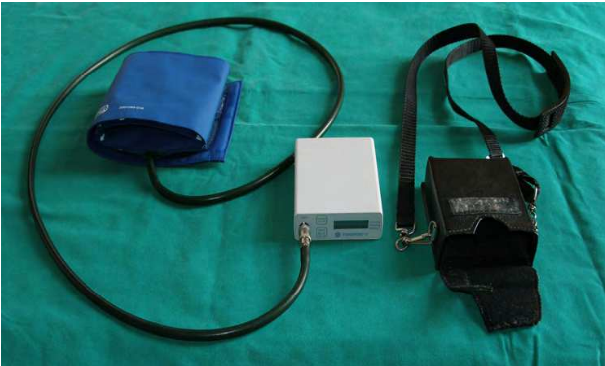
Fig. 2. CardioSoft – Tonoport – V – General Electric, USA device used for 24-hours ABPM
