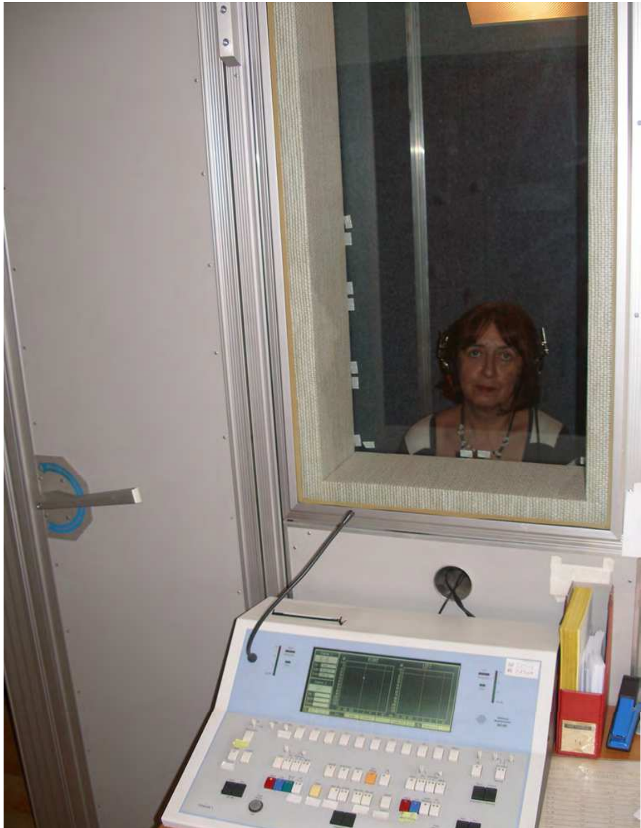
Fig. 1. Clinical Audiometer AC 40, Interacustics, Denmark used for measurement of thresholds of audibility and specification of tinnitus.
