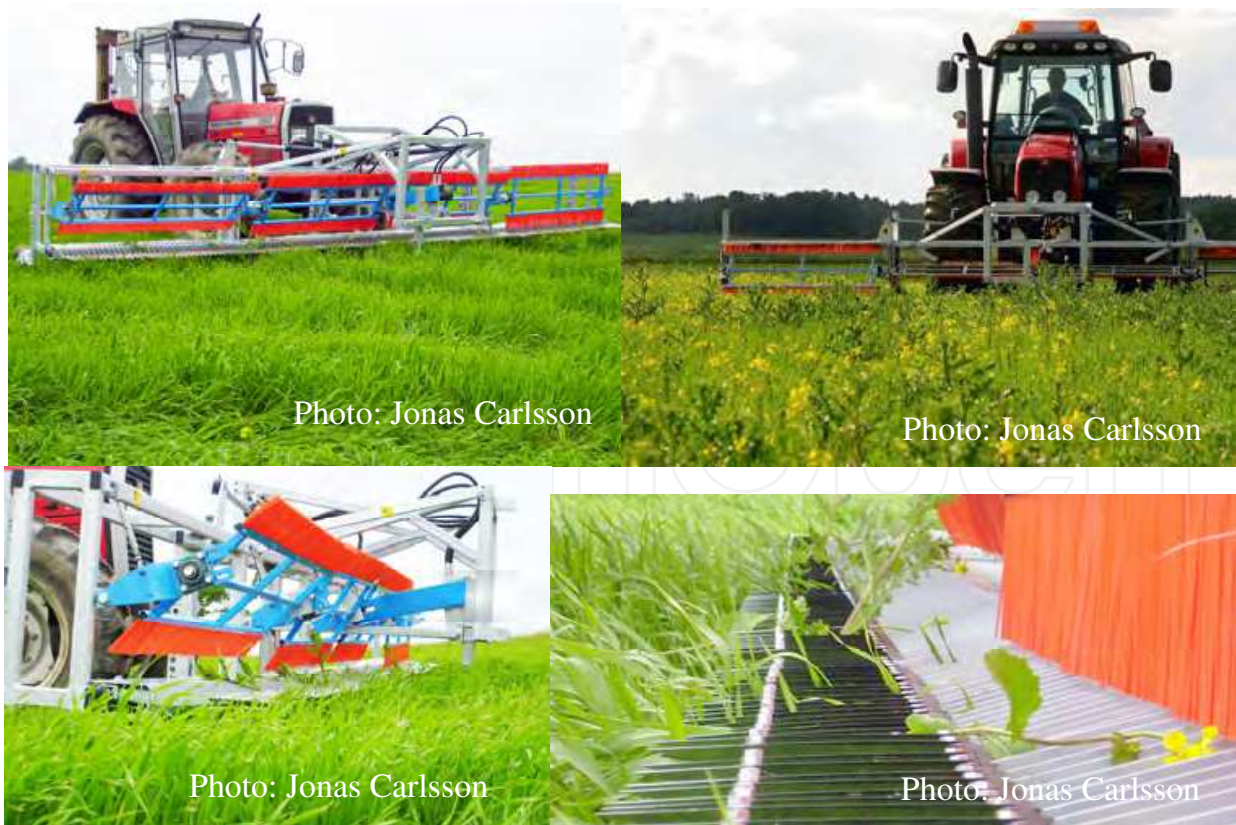
Fig. 7. Weed mower CombCut (upper left and right). Close up pictures of the brush reel (lower left) and the knives (lower right). Photo: Jonas Carlsson, JustCommonSense AB.
