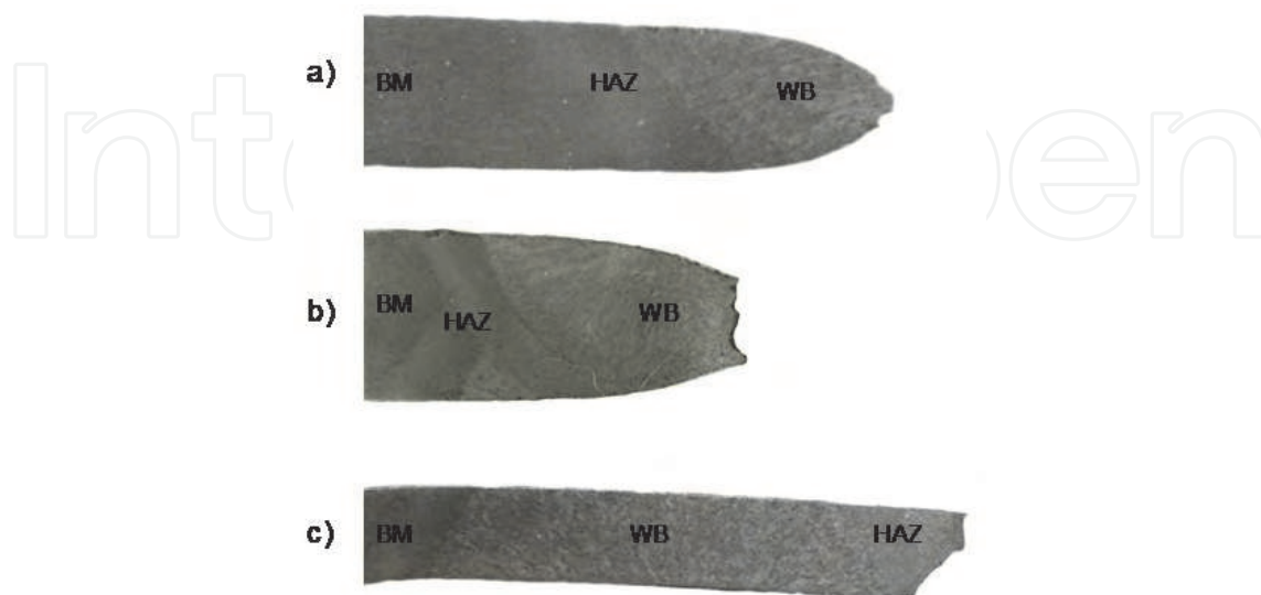
Fig. 4. Optical macrographs of the longitudinal sections (X70 steel) of the specimens after cracked, showing the zone where they failed: (a) tested in air, (b) tested in NACE solution at 25°C and (c) tested in NACE solution at 50°C
