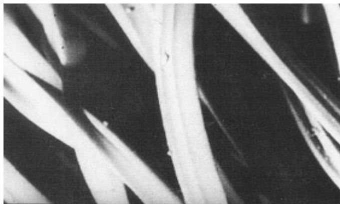
Fig. 2.2. SEM of treated polyester fabric with ethoxide (16) .
