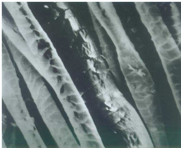
Fig. 1.3. SEM graph of sulphamic acid-treated wool.
