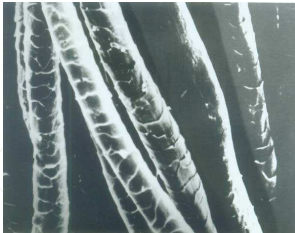
Fig. 1.2. SEM graph of untreated wool.
