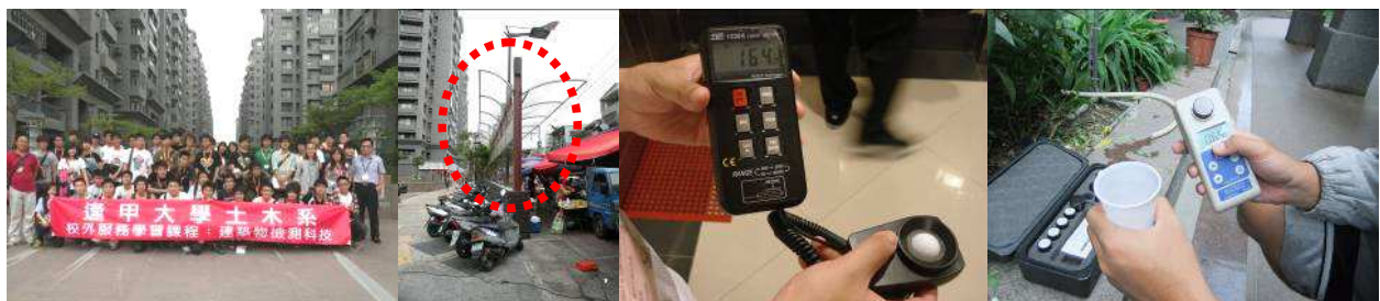
Fig. 16. The author led students to perform noise tests on sound-proof walls, illumination tests in stairways, and turbidity test on public use water
