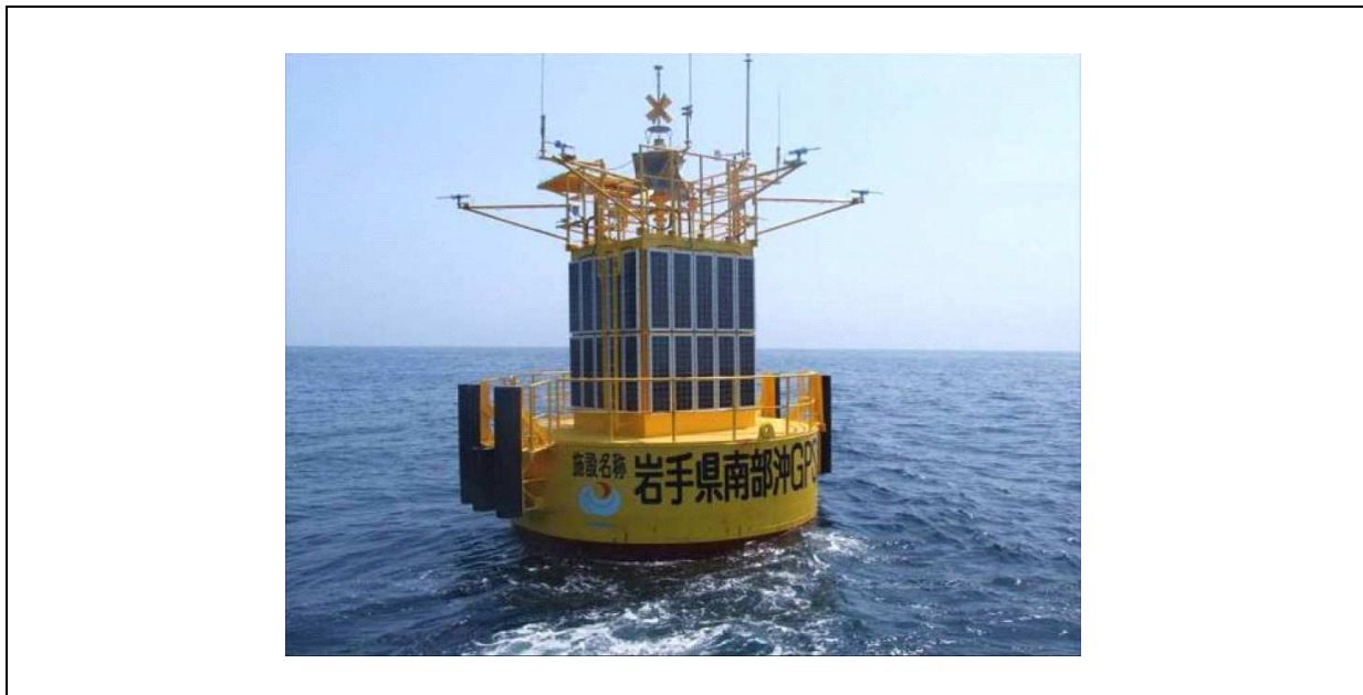
Fig. 4. Kinematic GPS buoy deployed offshore of NE Japan (photo by Port and Airport Research Institute).
