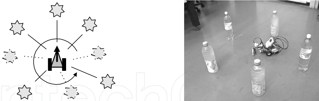
Fig. 3. The mobile robot with ultra-sonic sensor acting in the stochastic environment: after collision, the obstacle randomly changes its location in the environment.
