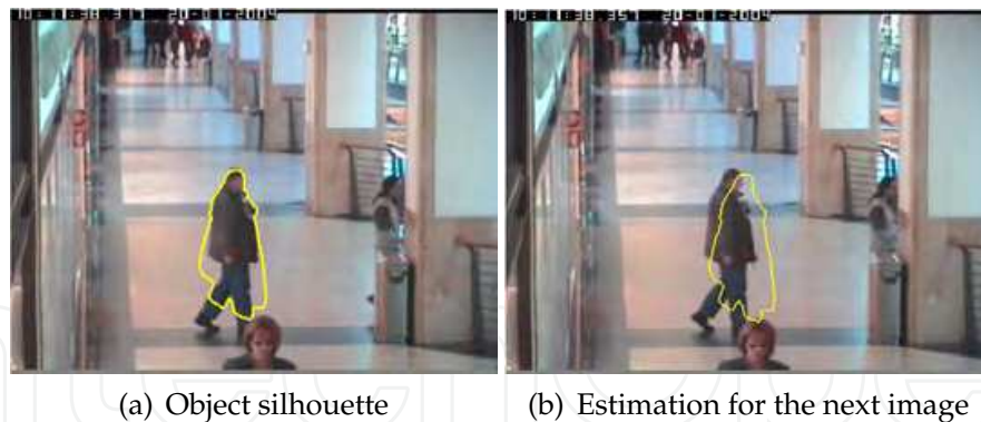
Fig. 11. Motion estimation using Kalman filter. a) The barycenter location at image t is used for predict its position at the next image. b) The irregular contour is centered at the predicted barycenter position, this will be used as initialization region in incoming images.
