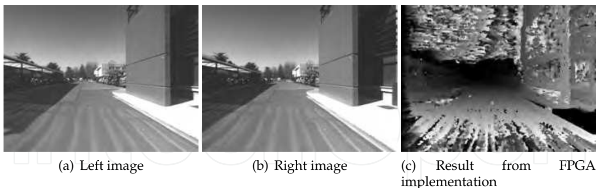
Fig. 3. Stereo images acquired from a mobile robot during outdoor navigation: a) left image b) right image and c) the disparity map.
