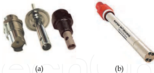
Fig. 2. 2-electrodes (a) and 4-electrodes (b) conductivity sensors.
