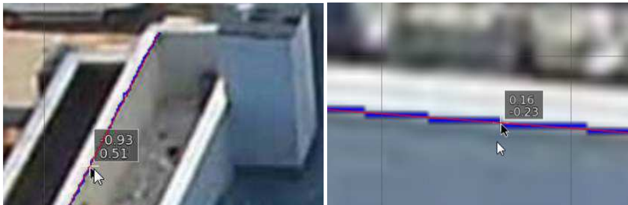
Fig. 2. AR-CAD line selection. A red line shows the line computed from the blue border pixels detected near the mouse. A white cross and a black pointer show the final pointer position (left). The result of the line selection process for a low resolution augmented image (right).
