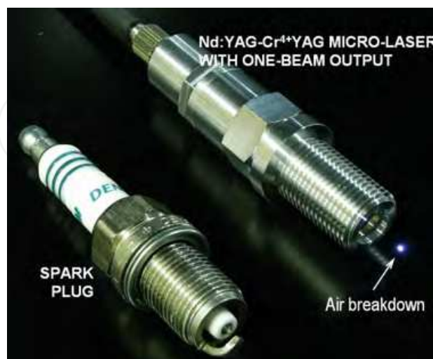
Fig. 9. Nd:YAG-Cr 4+ :YAG laser with one-beam output. Nd:YAG gain medium and Cr 4+ :YAG SA were single crystals; all optical components (including the output mirror) were discrete elements. Air breakdown is shown and size comparison is made with a spark plug.
