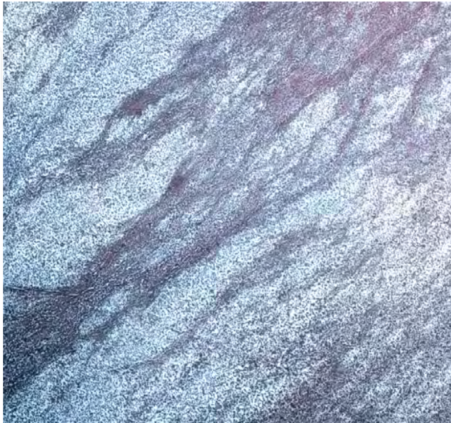
Fig. 6. Aerial photograph over the Jornada in October 2006 showing runoff flow paths after rainfall events at 25 cm resolution. Flow paths are darker because of an increase of surface soil moisture following overland flow.
