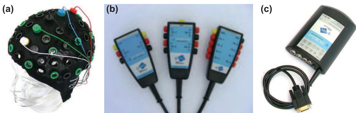
Fig. 7. EEG acquisition devices: (a) cap with electrodes, (b) connector and/or multiplexer, and (c) preamplifier.
