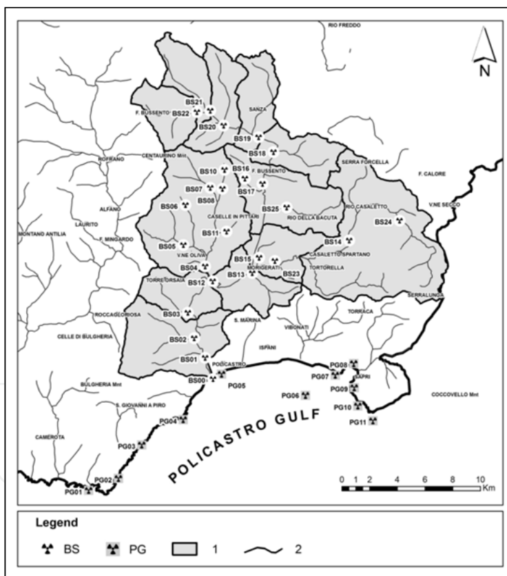
Fig. 4. The Bussento river basin monitoring network. BS is the symbol for streamflow stations whereas PG is the symbol for marine stations, for discharge and radon measurements.
