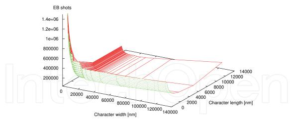
Fig. 6. The number of EB shots for Circuit 3
