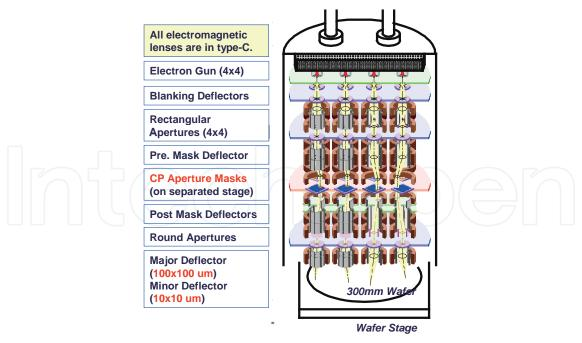
Fig. 3. An Advantest multi-column-cell character projection equipment
