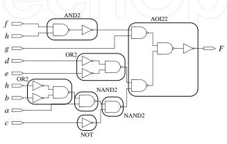
Fig. 9. A technology mapping result
