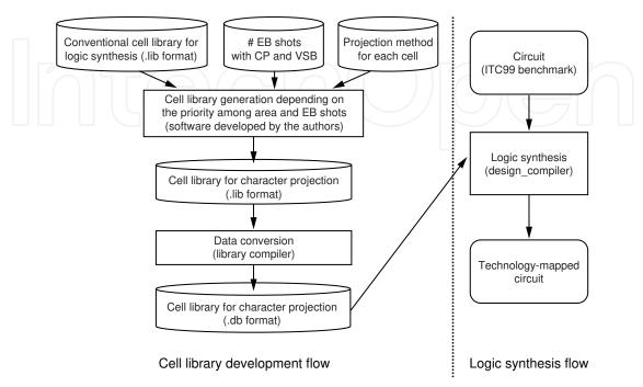
Fig. 11. Design flow in our design framework
