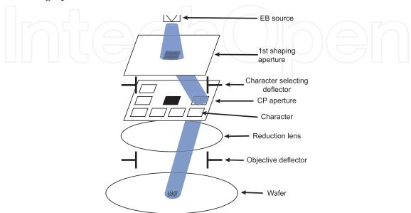
Fig. 2. Single-column-cell character projection equipment
