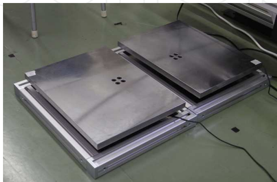
Fig. 5. Force detection plates for measuring feet pressure
