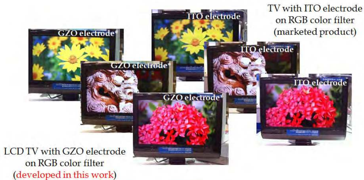
Fig. 14. Comparison of the display pictures between 20 inch LCD TVs with GZO and ITO electrodes on the RGB color filter.
