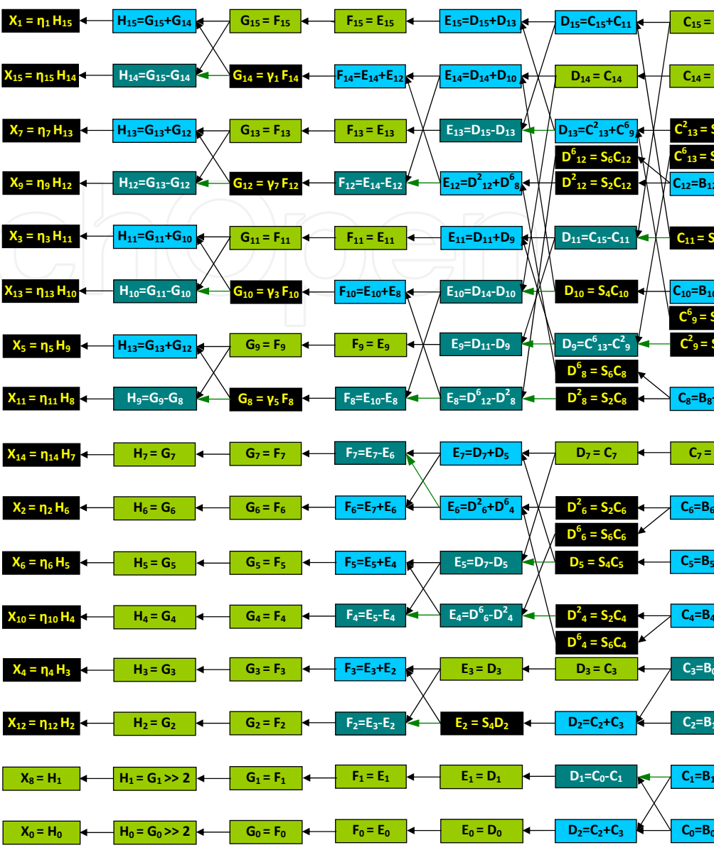
Fig. 8. The pipeline internal structure of 16-point DCT FPGA routine. Signal from the ADC propagates through the (horizontal) shift register x_{15}, \dots, x_0 . Simultaneously, the DCT coefficients are calculated in vertical chains in 9 clock cycles. Each rectangle corresponds to a single clock procedure (a logic block). 16-point DCT "engine" utilizes 35 multipliers, 45 adders, 32 sub-tractors and (16 + 38) shift registers. H_{0,1} = G_{0,1}/4 , a division is not implemented, two low significant bits are ignored. The width of data is extended in consecutive pipeline stages from N at the shift register x_{15}, \dots, x_0 , even to N+8 in the H routine.
