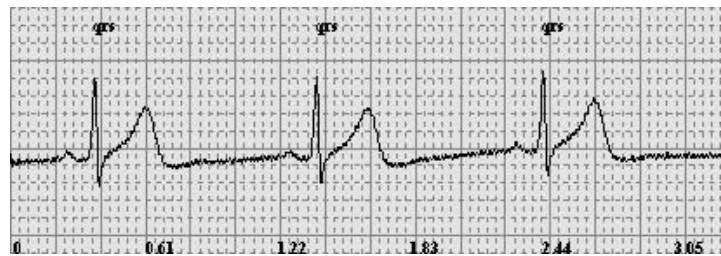
Fig. 19. Filtered ECG Signal Using Low-Pass 48 Hz Lynn's Filter
