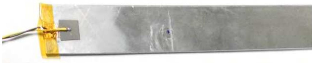
Fig. 1. A PZT patch bonded to an aluminum beam for damage detection.
