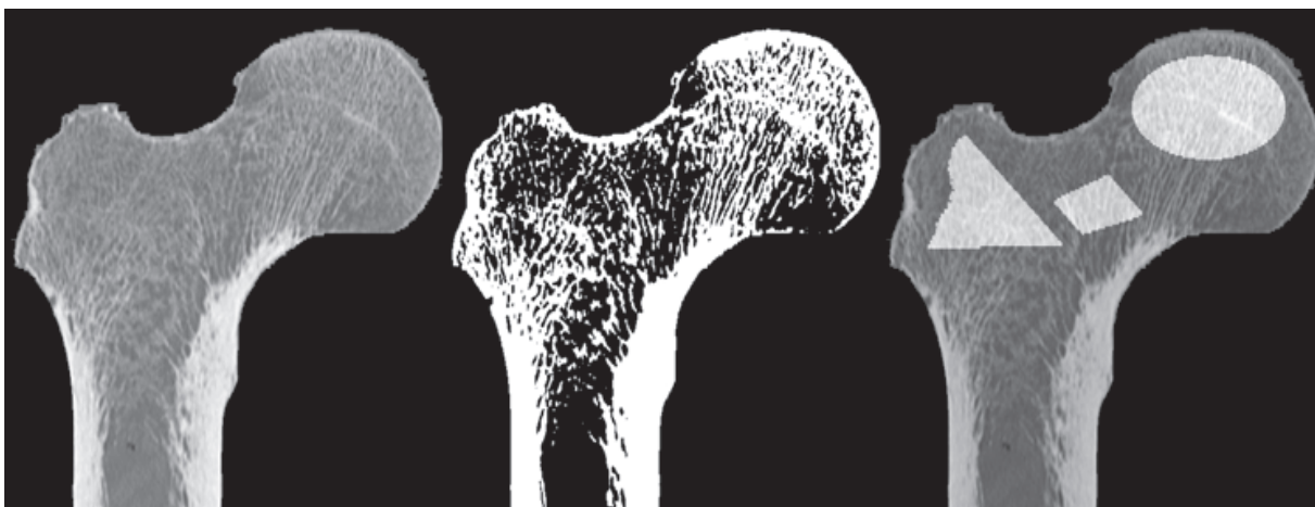
Fig. 1. Left: HRCT image of a human femur specimen with BMD = 0.69 \text{ g/cm}^2 and FL = 3912 \text{ N} (left). Middle: Binarized dataset according to the procedure explained in section 2.5. Right: Visualization of the fitted VOIs: head (ellipsoid), neck (cylinder), and trochanter (irregular) in the original CT data.
