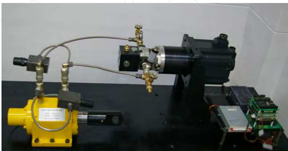
Fig. 6. Experimental setup of the EHA system
