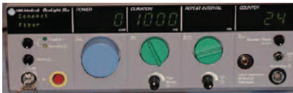
Fig. 2. Semiconductor Diode laser (IRIS Oculight SLx, Iris Medical Inc) for Diode contact TCP
