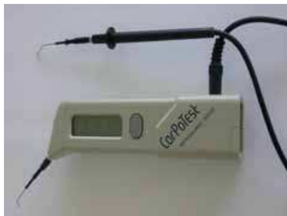
Fig. 7. Apparatus for measurement of corrosive potential.
