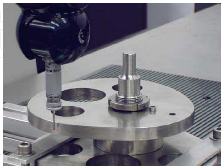
Fig. 8. Measuring the conjugate cam profiles by using a CMM
