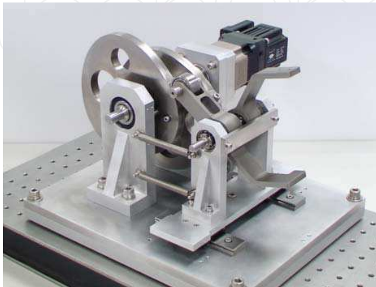
Fig. 6. Built assembled conjugate cams with measuring fixture
