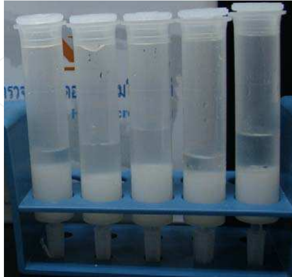
Fig. 5. DEAE Sepharose Microcolumn after preparation for hemoglobin E detection
