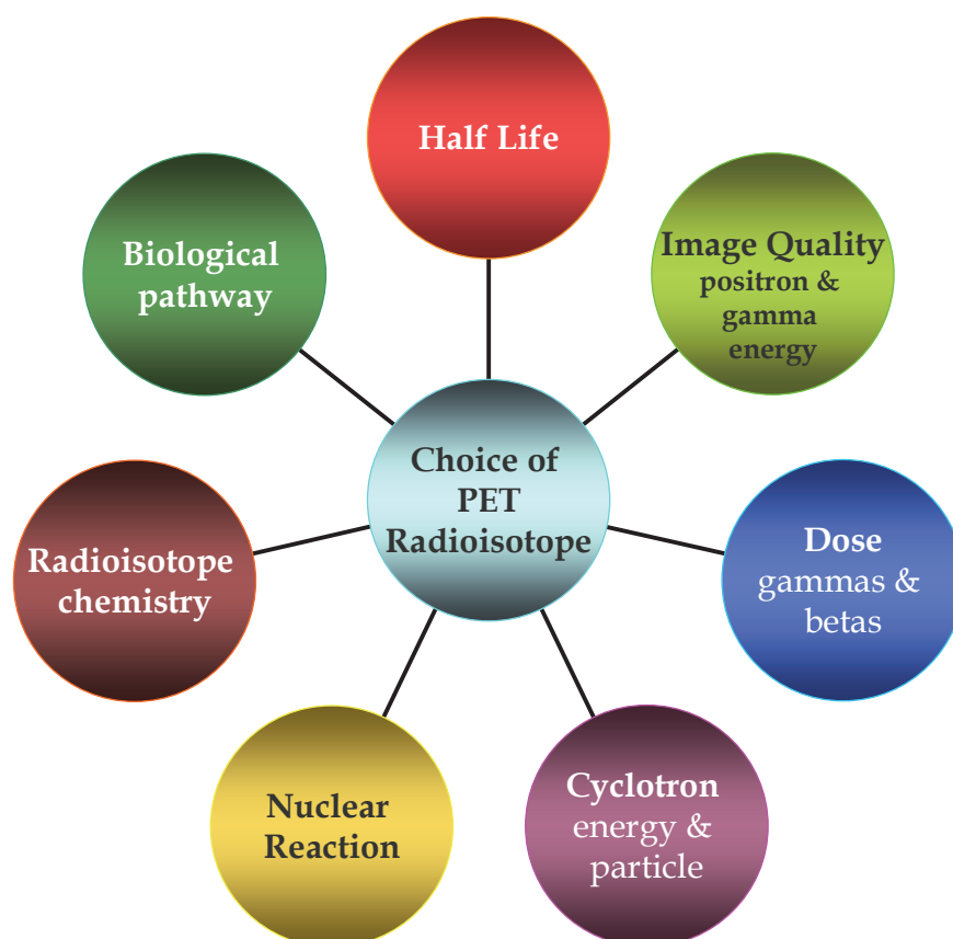
Fig. 2. Criteria governing selection of a PET radioisotope.
