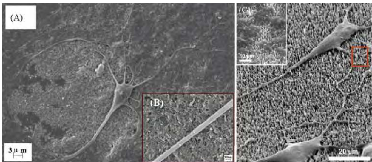
Fig. 2. a Neonatal hippocampal neurons adhering on purified multi-walled carbon nanotubes-coated glass substrates, showing extended neuritis after 8 days of culture; (B) single neurite in close contact to carbon nanotubes; (C) PC12 neural cells grown on vertically aligned carbon nanotubes coated with polypyrrole. Images from (Zhang & Webster, 2009). Reproduced with permission from Elsevier.
