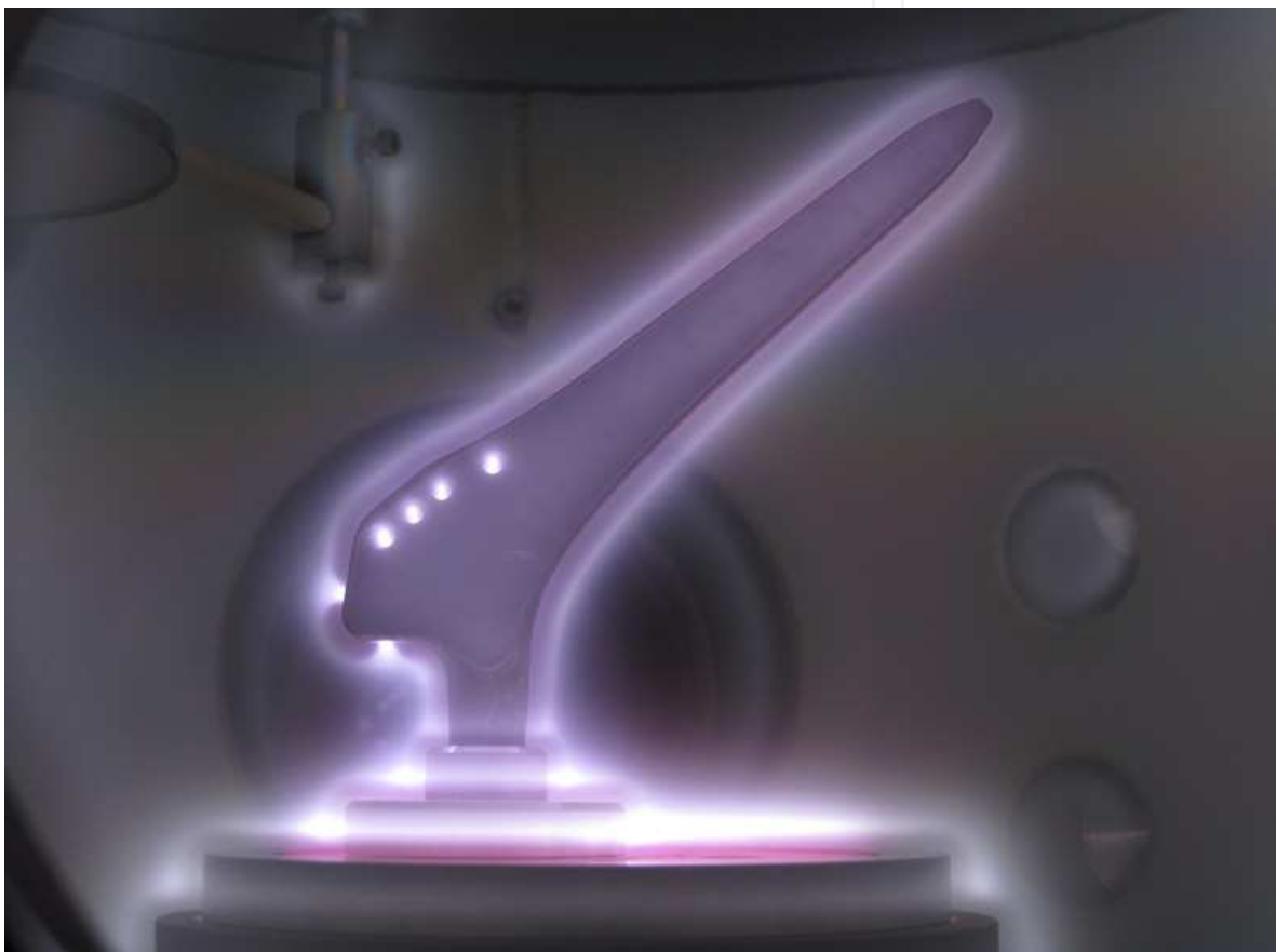
Fig. 2. Hip joint implant in low pressure plasma using a mixture of argon and ethylenediamine for cell adhesive coating
