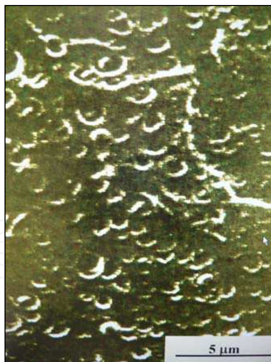
Fig. 3. Surface of COC-blend with designed pores with diameters ranging from 0.6 to 1.5 μm
