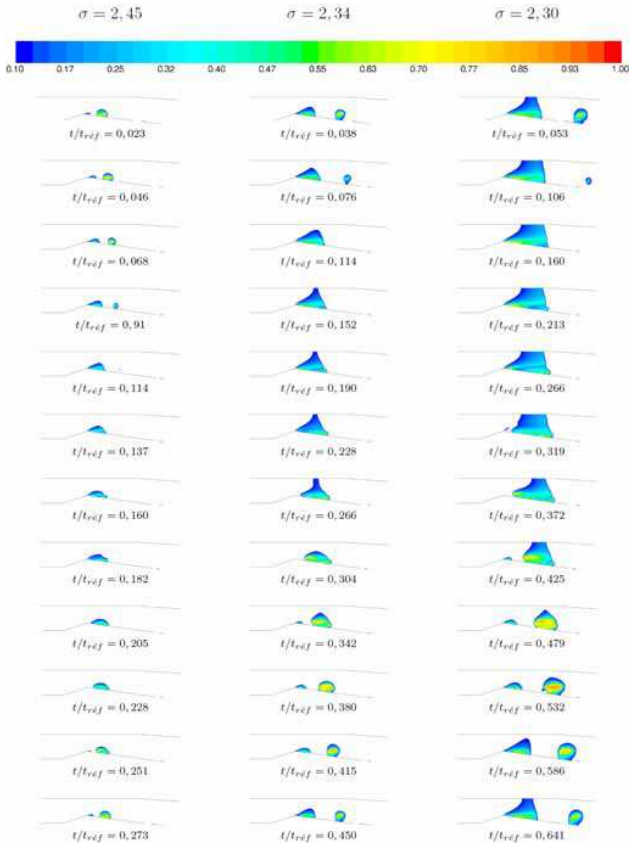
Fig. 4. Contours of vapour volume fraction ( a \geq 10\% ). Vapour detachment cycle calculated for three cavitation numbers. Calculations using RNG \kappa - \epsilon modified model, t_{ref} = 65.8E-3 s
