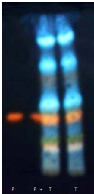
Fig. 6. TLC analysis of the tincture of Calendula officinalis L. Eluent I: ethyl acetate; formic acid; acetic acid; water (100:11:11:26); developer: NP/PEG 4000. Observation under light UV 365 nm; P- rutin standard ; T- Calendula tincture (Nunes, 2008; Nunes et al., 2009)
