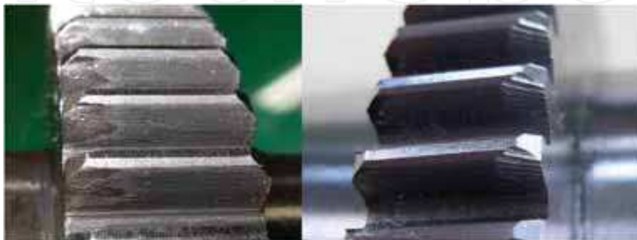
Fig. 8. Gear tooth weaned by misalignment
